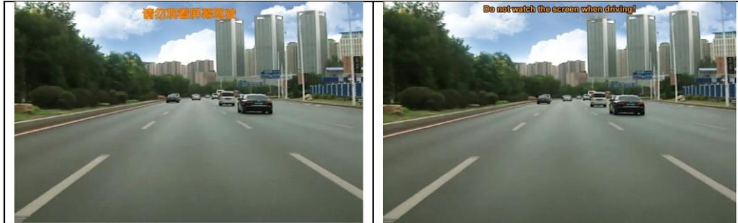
The warning sign of the LDW function will be shown as below. The sign shows that the vehicle will depart from the right side of the lane line. If the vehicle departs from the left side, the warning sign will be shown on the top left corner and the sign will be symmetric to the right side.
